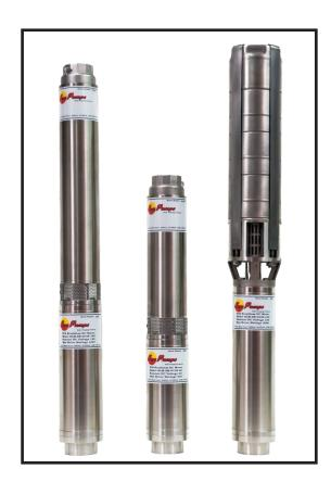
**SunPumps** SCS series submersibles are high quality, maintenance-free, DC powered pumps specifically made for water delivery in remote locations. They operate on 150 to 3000 watts of DC power with voltage choices ranging from 24 to 240 volts.
