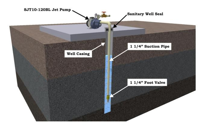
Figure 2 Typical Shallow Well Pump Installation
